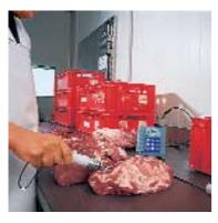
For applications where the object of measurement is particularly hard, firm or tough, such as is the case in a pH spot-check of raw ham, we advise the use of our **rugged puncture knife**. In combination with the puncture electrode and the pH meter 1120 or 1140, you have a sturdy measuring system to hand which is in a class of its own.
