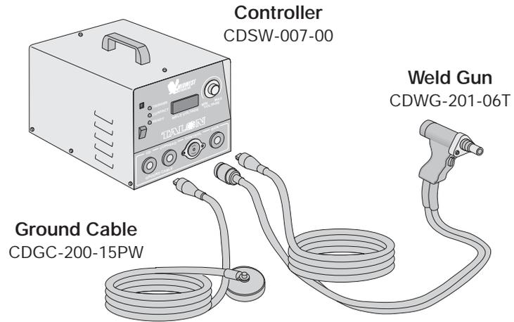
1. Carefully remove the controller, cables and weld gun from the shipping packaging.
