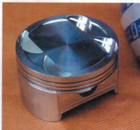
For motorsport, use forged pistons such as this from Omega
