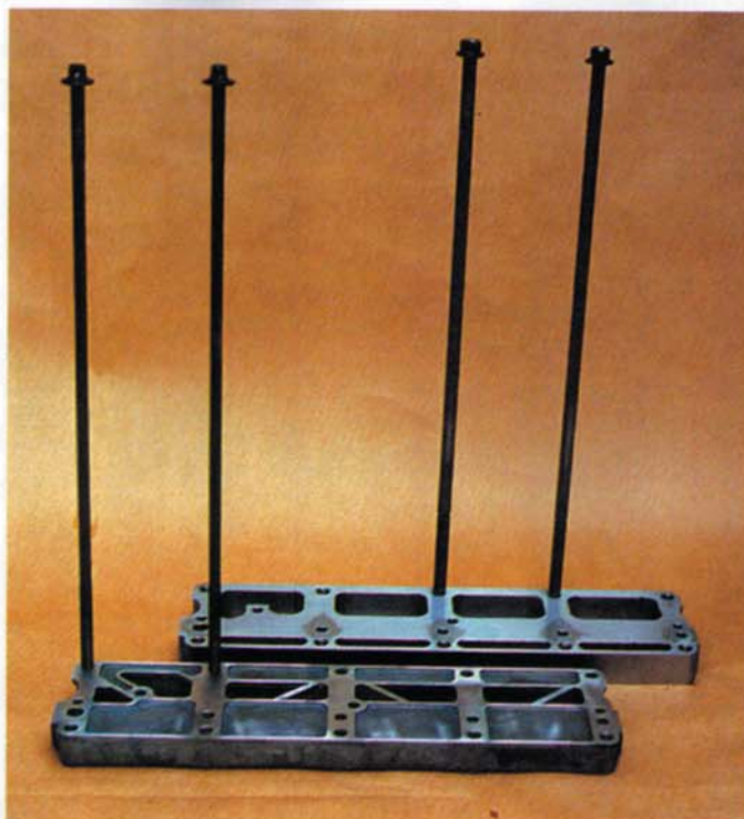
Comparison between original oil rail and longbolts and aftermarket replacements (behind) which can be used to cause crank binding and fatigue failure of the block
