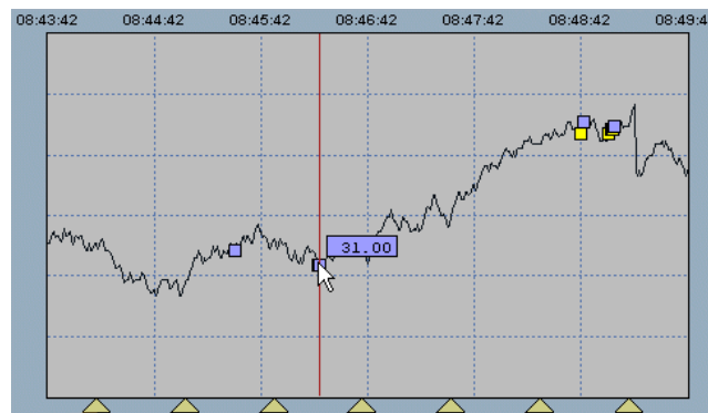
Figure 6: Trend diagram with events. The events visualised by the rectangles are related to the trended variable and its position follows the curve. The triangles at the bottom visualise events with relation to time only.
